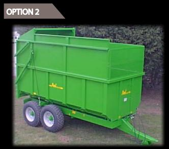
Standard silage kit plus full front mesh panel and reversible extra side panel (used in conjunction with canopy)
