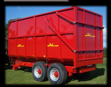
The full panel silage rear door has the same rigid RHS framework fitted with a full solid panel as shown above.
