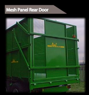
The standard silage rear door has a rigid RHS framework, a solid centre panel with mesh either side as shown above. (The flashing beacon shown is available as an optional extra.)
