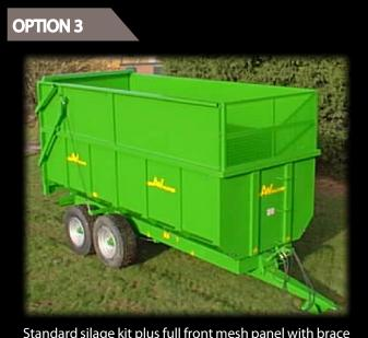
Standard silage kit plus full front mesh panel with brace bar (in lieu of canopy)
